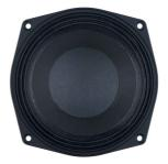
The MBX series mid-bass woofers from B&C Speakers offer acoustic designers a new range of high efficiency, wide bandwidth alternatives that are not currently available in the B&C range. These full-featured transducers incorporate lightweight neodymium motors, inside/outside wound copper clad aluminum wire voice coils, weatherproof impregnated paper cones, and a symmetrical inductance profile. The MBX Series is especially well suited for two-way loudspeaker enclosures.
